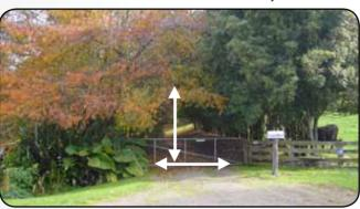
Above: Emergency service vehicles like ambulances and fire trucks need at least a four metre clearance in terms of width of driveway (fence/gate posts and vegetation) and height (vegetation and overhanging trees).
